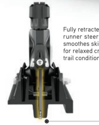
Fully retracted, the Pilot TS runner steers easily and smoothes ski tracking. Best for relaxed cruising and icier trail conditions.
